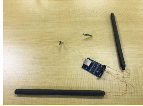
Fig. 8. H-field antenna (20 cm ferrite antenna)
