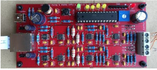
Fig. 4. Magnetic field amplifier (Red system)
