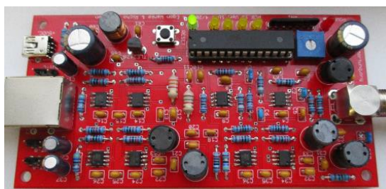
Fig. 3. Electric field amplifier (Red system)
